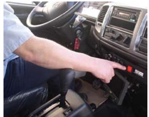
The HTS uses a dash release button with a flashing light and audible alarm to warn the driver if the hand truck is not locked in the Ultra-Rack. Also has a manual key override on the Ultra-Rack frame.
